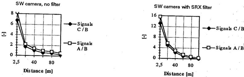
Fig. 5 Influence of the signals from the atmosphere („B”) to the signals detected from sources „C” and „A” (temperature of these sources was 5 -8 K above the local temperature of the atmosphere)
