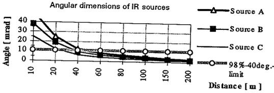
Fig. 2 Limitation of correct readouts caused by changes of the source's angular dimension
