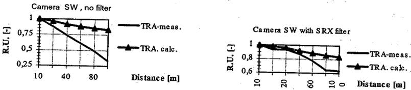
Fig. 6 Coefficients of the atmospheric transmission estimated in accordance with equation (5) for „TRA-meas.” curve and equation (6) for „TRA calc.” curve (based on experiment and ERIKA program respectively)
