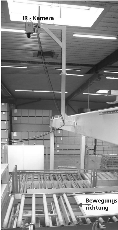
Fig. 5. Thermographic set-up just behind a paper laminating press. By moving the material along the infrared-camera possible defects can be detected.
