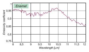
Fig. 2. Emissivity coefficient of the enamel
