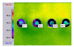
Fig. 1. Apparent temperature distribution of dental materials
