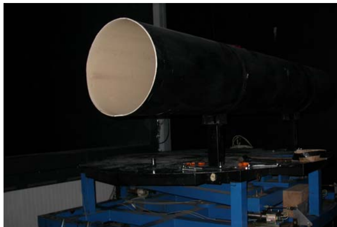
Figure 9: Cylinder installed in the wind tunnel
