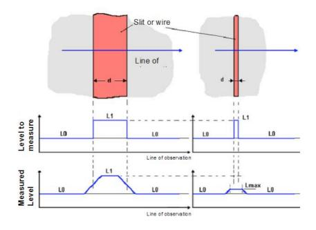
**Fig. 2b.** Slit Response Function. Below a certain value of *d*, the  $L_{max}$  value of the thermosignal decrease from  $L_1$  to  $L_0$  (figure is issue from reference 4)
