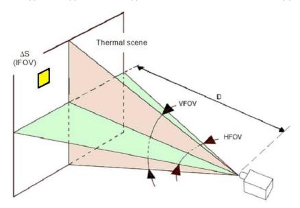
Fig. 1. angles HFOV. VFOV and IFOV (figure is issue from reference [4])
