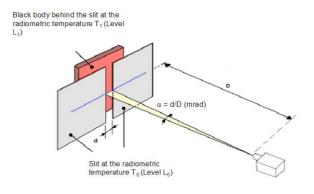
**Fig. 2a.** Slit Response Function. Camera sees slit lips of radiometric temperature  $T_0$  (back side radiometric temperature) and The body behind the slit of radiometric temperature  $T_1$  ("slit " temperature). Slit width is d and D is the distance slit-camera (Figure is issue from reference 4)
