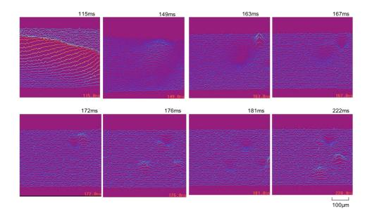
*Fig. 4.* Three dimensional (3D) plot of differential image of IR thermographs of the latent heat from a single tobacco cell during freezing.
