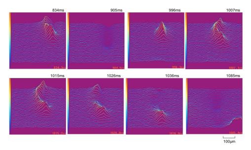
*Fig 2.* Three dimensional (3D) plot of differential image of IR thermographs of the latent heat from a single onionskin cell during freezing.
