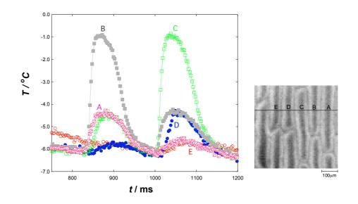
*Fig. 5.* Intercellular heat transfer of the latent heat of onionskin cells during freezing affects the temperature-time profile in the individual cells.
