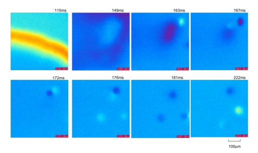
**Fig. 3.** Differential image of IR thermographs of the latent heat from a single tobacco cell during freezing.
