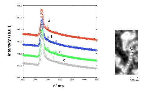
**Fig. 6.** Intercellular heat transfer of the latent heat of the cultured tobacco cells during freezing in the medium affects the temperature-time profile of the onedimensionally linked individual cells.
