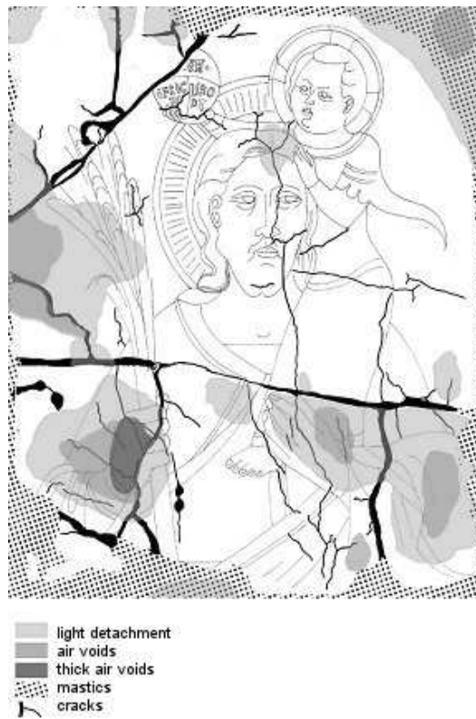
Fig. 16. : Results obtained by acoustic sounding
