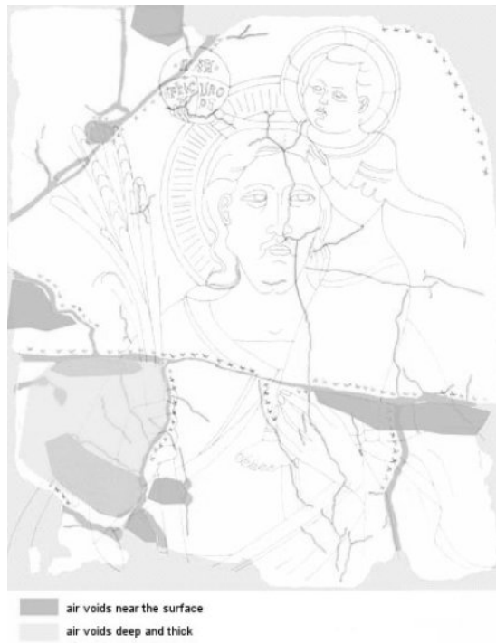
Fig. 15. : Results obtained by photothermal radiometry
