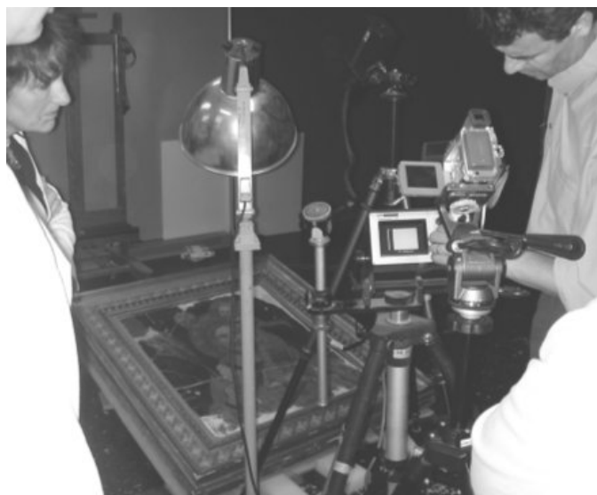
Fig. 8. : Non destructive testing of the Saint Christopher by infrared thermography : The experimental device
