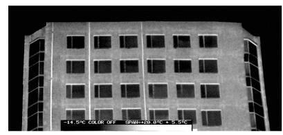
*Fig. 10* Negative Building Pressure (-60 Pa),  $T_o = -7^{\circ}C$ , maintained for a duration of 4 hours prior to inspection.
