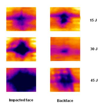
*Figure 3* Typical IR thermography images of impacted areas in 3-D commingled laminates (40x32 mm area) (all of these images were acquired after 15 seconds transient)
