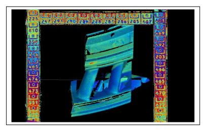
*Fig 9:* Image of the 3d point cloud textured with the thermographic data image 7, using pixel rays. This technique is similar to the ray tracing methods
