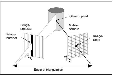
Fig 2: Principle of fringe projection
