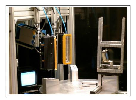
**Fig 6:** The thermographic equipment, the specimen and the cage. The infrared camera also records the optical marks. Since this camera is photogrammetric calibrated it is possible to calculate the position of the camera relative to the cage.
