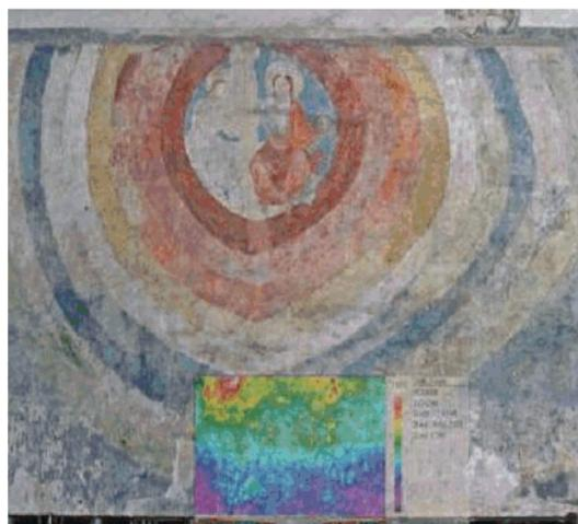
Fig. 19. Gothic painting in church of Lady Mary in Torun, thermal image show the distortion of bottom part of the painting, paraffin and soot from the candles being lighted for years
