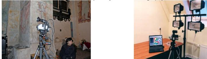
Fig. 7. Thermal system for dynamic investigation in gothic churches
