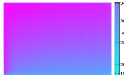
Fig. 5. Differential thermogram of the frontal surface of the investigated heater ( t_1 = 60\text{ }^\circ\text{C} , q_v = 30\text{ l/h} )
