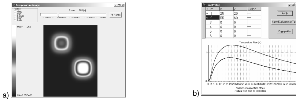
Fig.3. Theoretical temperature evolutions over moist polyurethane foam (volumic microwave heating, monitoring gypsum, ThermoCalc-6L): a – temperature distribution at 160 s, b – temperature evolutions (2 g H 2 O – bottom plot, 4 g H 2 O – upper plot)
