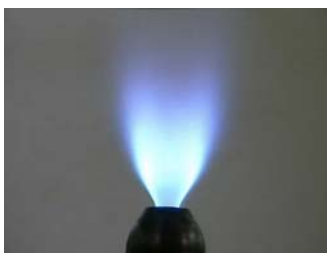
Figure 1. Typical picture of a lean flame (AFR=25, frame rate 50 f/s).
