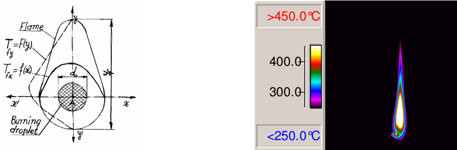
Fig. 3. Flame detail with schematically representation at DFMV, of a superior gas oil GO droplet and IR thermogram for the some fuel droplet ( d_0 = 1.7\text{mm} , T_e = T_0 = 295\text{K} ) at DFMV
