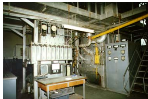
Fig.5 : Pilot installation of 2MWt used to test the combustion process of paper refuse (1) Cold air ventilator ; 2) Post combustion grate ; 3) Visit hole ; (4) Main burner ; (5) secondary waste bunker ; (6) Secondary feeding installation ; (7) Secondary feeding orifice ; (8) Tubular air preheater ; (9) Main air ventilator ; 10) Flying ash separator ; (11) Flue gas ventilator ; (12) Burning chamber ; (P10) – natural gas injection.
