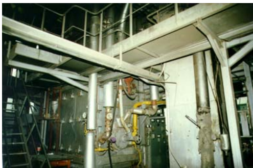
Fig.5 : Pilot installation of 2MWt used to test the combustion process of paper refuse (1) Cold air ventilator ; 2) Post combustion grate ; 3) Visit hole ; (4) Main burner ; (5) secondary waste bunker ; (6) Secondary feeding installation ; (7) Secondary feeding orifice ; (8) Tubular air preheater ; (9) Main air ventilator ; 10) Flying ash separator ; (11) Flue gas ventilator ; (12) Burning chamber ; (P10) – natural gas injection.
