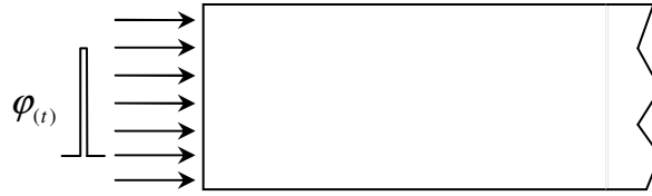
Fig. 1. Semi Infinite body thermal model as used in the DAC or EC ISIB
