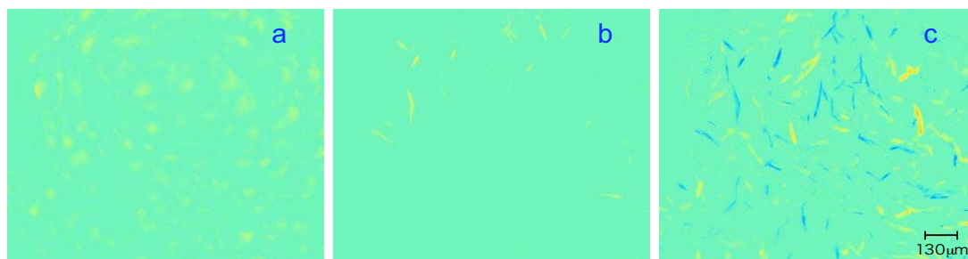
Fig. 8 Differential images of exothermic heat pattern in (a) crystallization, (b) rotator phase transition in cooling ( -20^{\circ}\text{C}/\text{min} ), (c) rotator phase transition in heating ( +20^{\circ}\text{C}/\text{min} ) of \text{C}_{23}\text{H}_{50} .
