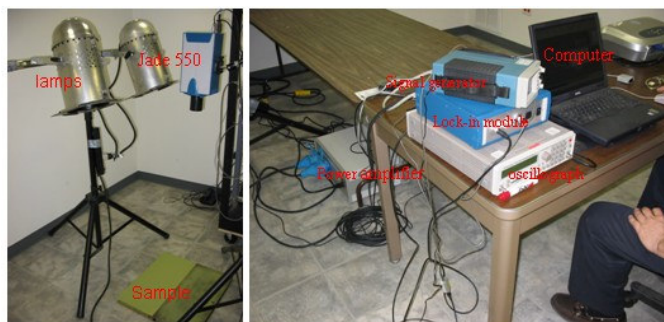
Fig. 2. Cedip JADE MWIR 550 Lock-in thermography system
