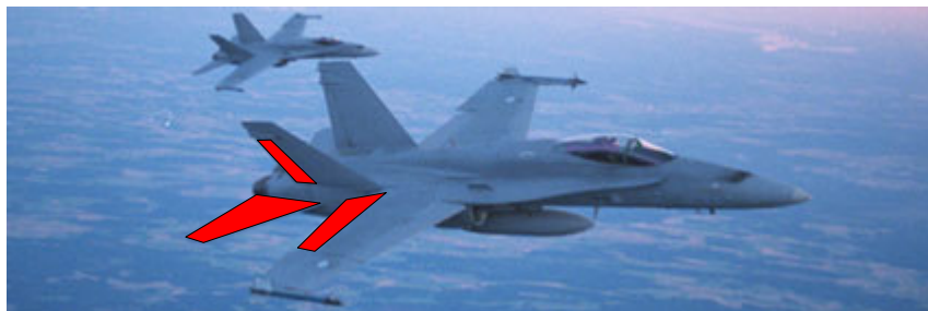
Fig. 1. The moisture detection areas under investigation (port and starboard side of the aircraft). Red indicates the interest area of flight control surfaces (rudder, trailing edge flap and horizontal stabilizer). Courtesy of the FIAF.
