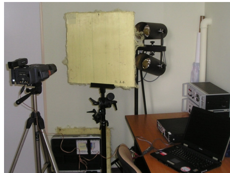
Fig. 5. Measuring station for non-destructive testing using active thermographic technique
