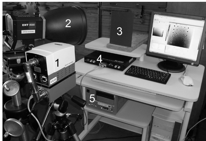
Fig. 3. Experimental set-up for pulse thermography: 1 – IR camera, 2 – flash lamp, 3 – tested specimen, 4 – interface between IR camera and excitation lamp, 5 - computer.
