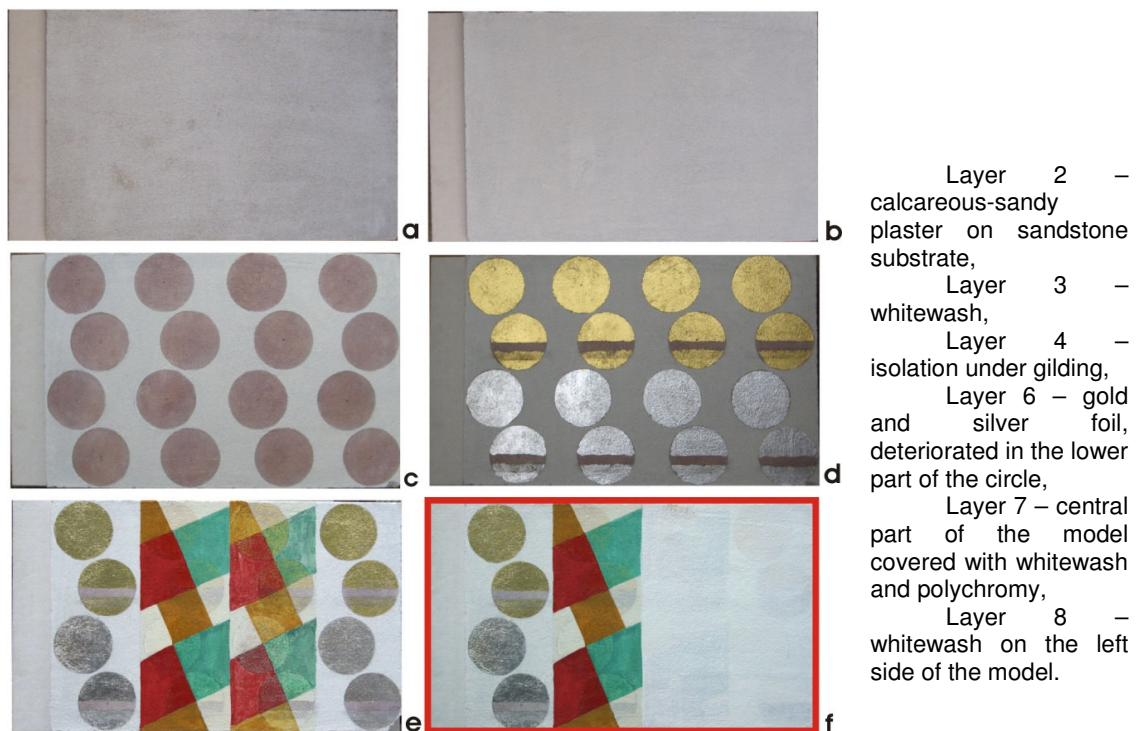
Fig. 2. The stages of model construction, layers marked as on model cross-section
