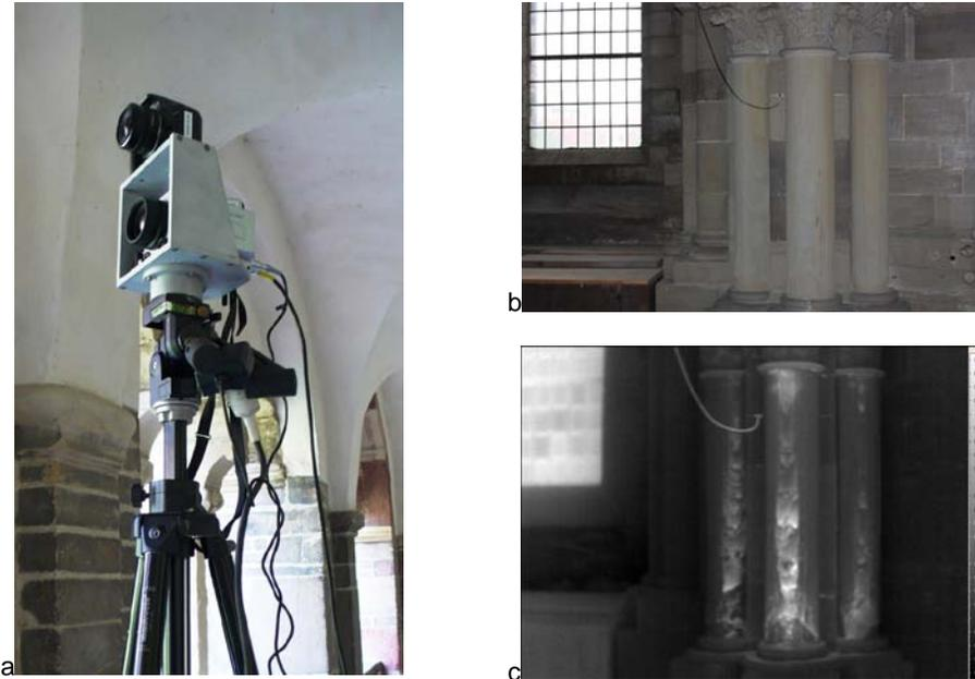
**Fig. 1.** a: Frame for CCD camera and IR camera for the determination of extrinsic calibration parameters; b: Photo; c: Thermogram from sandstone column described below.
