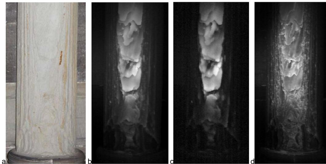
**Fig. 3.** Bottom part of a sandstone column with spalling in June 2009. a: Photo; b: Thermogram, directly recorded after a heating time of 60 s with two halogen lamps (10.6 to 18.0 K from black to white). c: Amplitude image at 0.02 Hz calculated by pulse-phase thermography after 60 s heating; d: Amplitude image calculated from lock-in thermography at 0.05 Hz.
