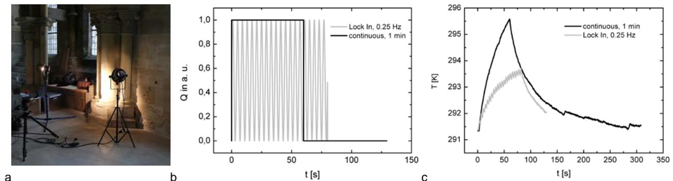
**Fig. 2.** a: Illuminated (heated) bottom part of a sandstone column; b: Heat flow as a function of time for impulse heating for 1 min (black curve) and periodic heating with a frequency of 0.25 Hz; c: Average temperature at the middle of the column as a function of time during and after heating.
