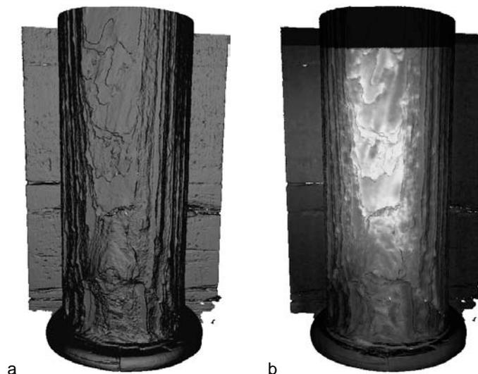
**Fig. 5.** a: Visualized surface of the column recorded with the 3D laser scanner in June 2009. b: Data fusion of geometrical 3D data and amplitude image recorded in June 2009 with a frequency of 0.05 Hz.
