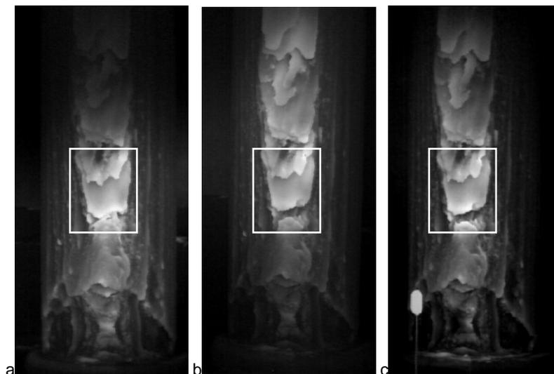
**Fig. 4.** Thermograms directly recorded after a heating time of 60 s with two halogen lamps at different seasons; a: June 2009 (18.0 to 23.3°C from black to white); b: November 2009 (10.6 to 18.0°C from black to white); c: March 2010 (9.4 to 14.4°C from black to white). The white rectangle marks the area with considerable loss of material.
