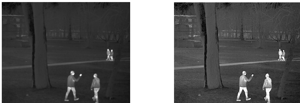
Fig. 11. Thermal images: original (left) and processed by image enhancement algorithm (right)
