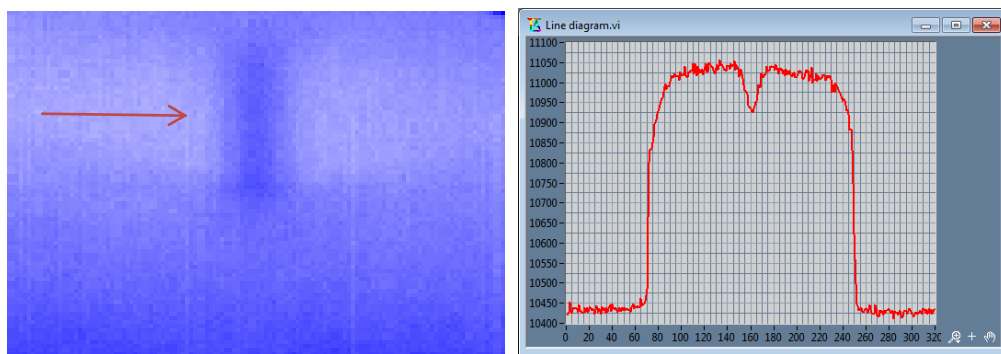
Fig. 5. Left: Thermographic image of a mild steel plate at a frequency of 300 Hz. A defect indication from an artificial hidden defect at a depth position of 1.25 mm with a length of 10 mm is visible (image size about 40 mm x 30 mm). Right: signal profile (in digital levels) along the arrow in figure 5, left.
