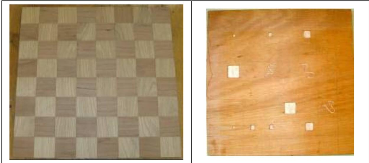
Figure 6: Analyzed marquetry and the position of the delaminations and of the galleries of worms
