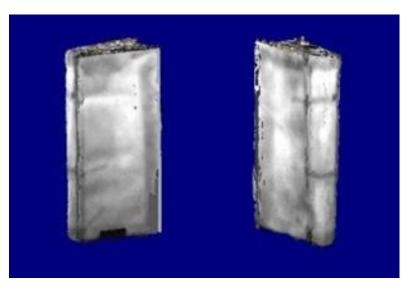
Fig. 2 - 3D thermographic recostruction of a seventeenth century volume.
