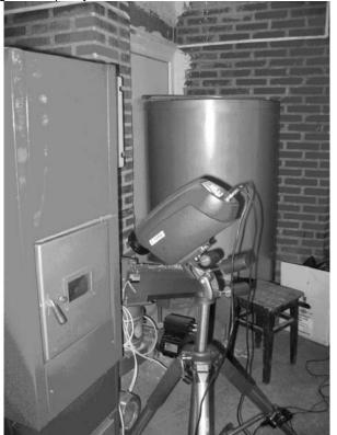
Fig. 6. Test boiler for shredded sorghum equipped with infrared monitoring system
