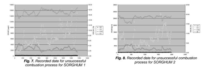
The NOx concentration values are very low due to the very low values of recorded temperature. By contrast, the carbon monoxide concentration has been very high – exceeding the apparatus range of 10000 ppm. At the same time, very reduced values of carbon dioxide concentration have been recorded in opposition to very high oxygen content in the flue gas. The corrected infrared image of the furnace also indicated a range of low flame temperature values (Figure 9).
