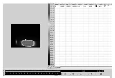
Fig. 12. Infrared image for normal temperature values in case of normal combustion process.
