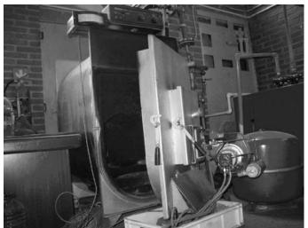
Fig. 2. PIFATI boiler of 55 kW - here both the liquid fuel burner and the grated solid fuel furnace can be seen together
