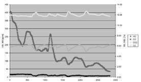
**Fig. 11.** Recorded date for flue gas composition in case of successful combustion process for SORGHUM 2
