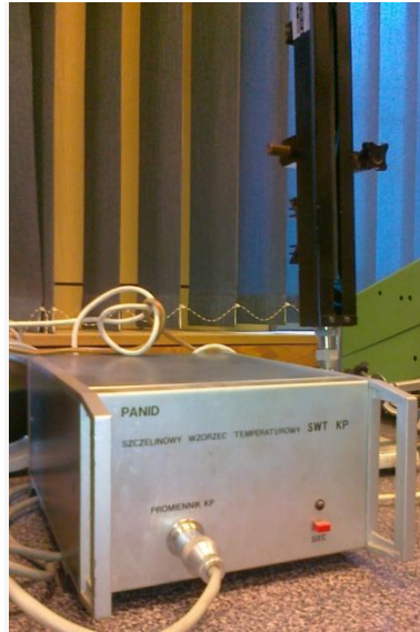
Fig. 4 The wire IR emitter with the pulse temperature controller
