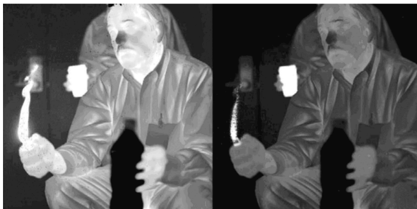
Fig. 14. An image taken with the first megapixel simultaneous pixel co-registered MWIR:LWIR dual-band QWIP camera. The flame in the MWIR image (left) looks broader due to the detection of heated \text{CO}_2 (from cigarette lighter) re-emission in 4.1–4.3-micron band, whereas the heated \text{CO}_2 gas does not have any emission line in the LWIR (8–9 microns) band. Thus, the LWIR image shows only thermal signatures of the flame.
