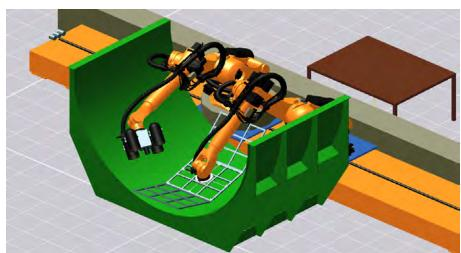
Fig 7 Approach - production integrated, automated Thermography
