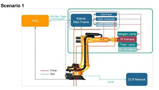
Fig 11 Scenario 1 - Control system mounted on robot arm, excitation and camera on hand
