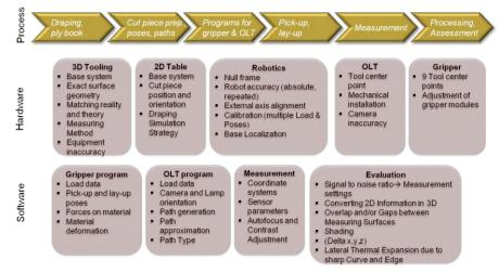
Fig 15 Control on process accuracy
