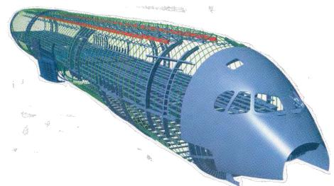
Fig 3 structural design of a fuselage with stringers, frames and beams (Source: Flugrevue A350XWB)
