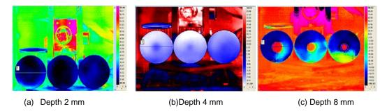
Fig. 3 Imaging's of Lock-in Thermography for SM20C specimens
