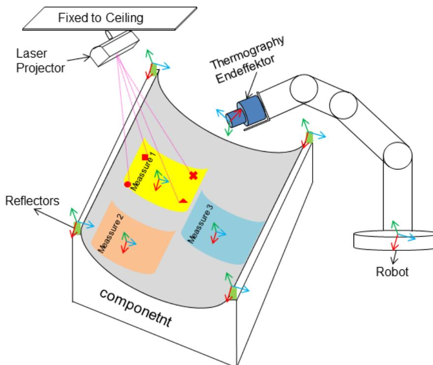
**Figure 10: Concept for measuring the position of robot guided workpiece**
