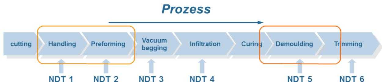
Figure 1: Schematic CFRP manufacturing process with inline NDT highlighted
