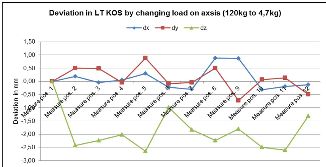
**Figure 5: Positions deviation influenced by loading in IQZ robot cell**
