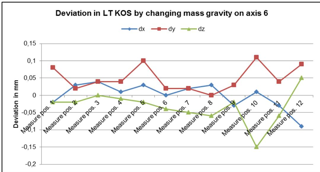
**Figure 4: Position deviation influenced by mass gravity in IQZ robot cell**
