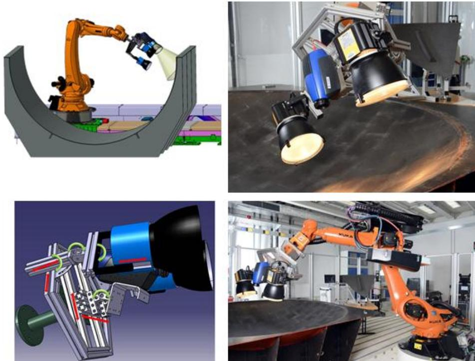
**Figure 3: Robotic end-effector mounted on industrial robot**
