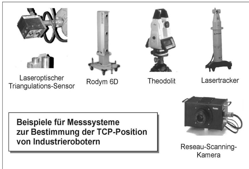
Figure 9: sensor based Measurement to improve the robot accuracy
