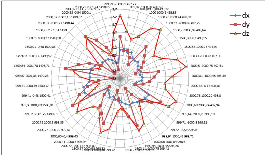
**Figure 6: Positions deviation influenced by external linear axis in TEZ robot cell**
