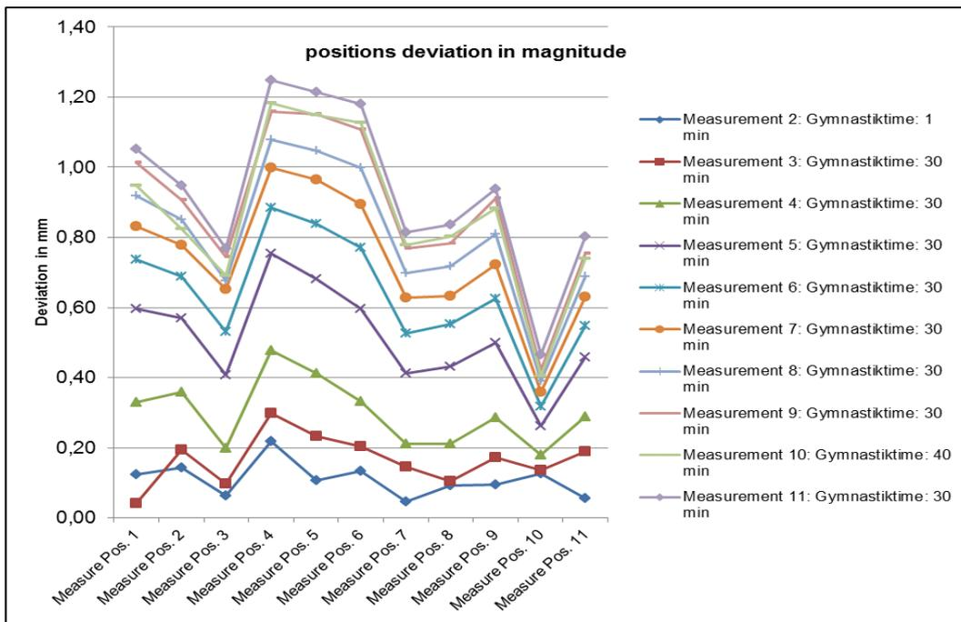
Figure 8: Position deviation due to temperature incensement
