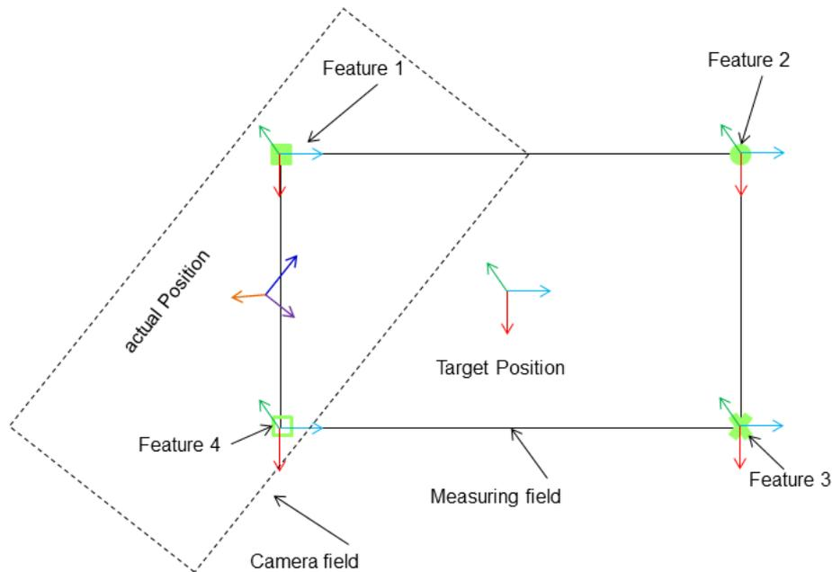
**Figure 11: Possible example of position deviation between robot target position and the robot actual position**
