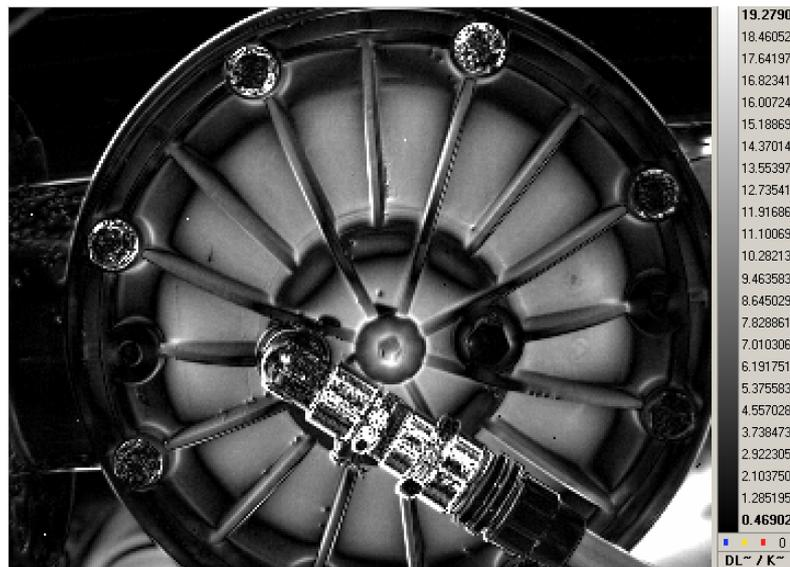
Fig.2. TSA image of the cover, when the valve is operated by the solenoid ( $\Delta P=3$  bar).
