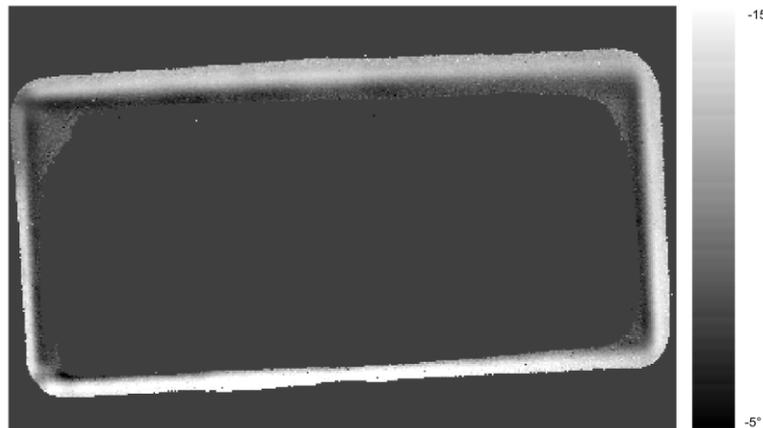
**Fig. 5.** Flying-spot lock-in phase image of the metal sheet sample
