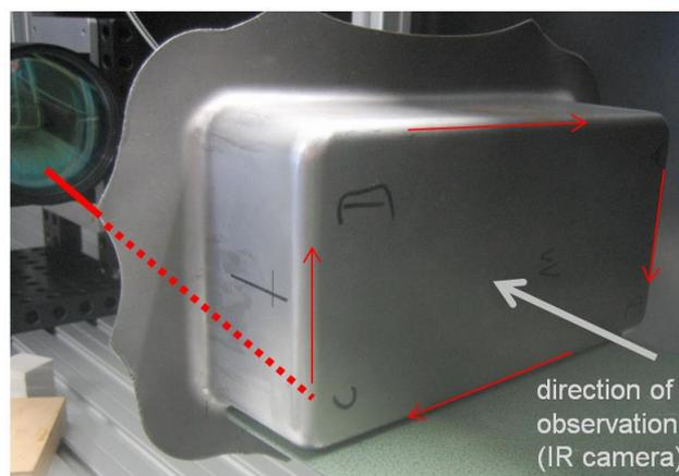
**Fig. 3.** Photo of a sample in the test setup. Excitation is performed from the rear side by rapid scanning of a laser spot along the inner side of the cup. On the left side, the lens of the scanning head is visible. The red arrows indicate the laser spot movement. Detection by IR camera is performed from the bottom side of the cup (thermal transmission)
