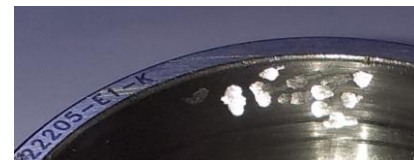
Fig. 3. Intentionally pre-damaged outer raceway
