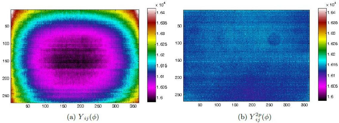
Fig. 4. a) Raw thermogram, b) thermogram a) corrected with the proposed method
