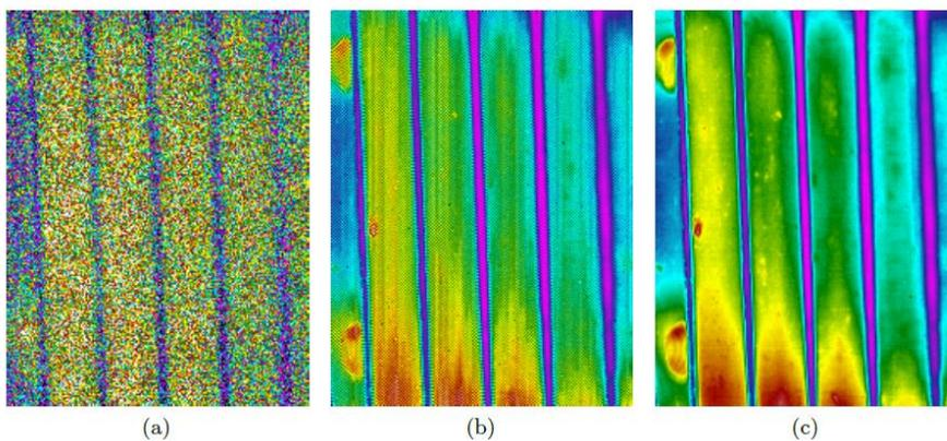
**Fig. 1.** (a) Exemplary thermogram before non-uniformity correction, (b) after one-point or (c) two-point non-uniformity correction.
