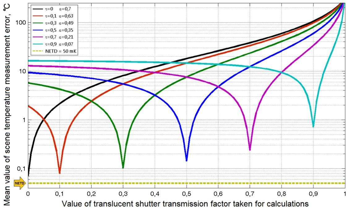
Fig. 5. Simulation of mean value of scene temperature measurement error versus the value of translucent shutter transmission factor taken by the user for calculations
