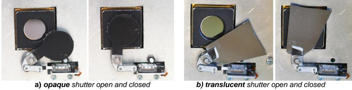
**Fig. 2.** Images of a) opaque and b) translucent shutter mounted inside the thermal camera
