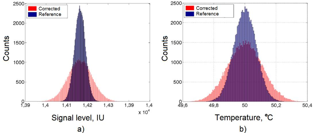
**Fig. 6.** Simulated exemplary histograms of corrected and reference thermograms for a) correction without frame averaging, b) 20 frames averaged in time domain
