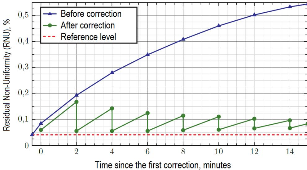
**Fig. 3.** Efficiency of the proposed method of thermal drift correction tested with blackbody model
