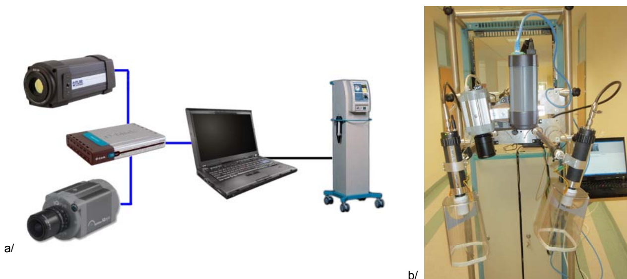
Fig. 1. The ADT set, a/ components: the data acquisition system, thermal and video cameras and a cryotherapy device for cooling excitation, b/ the laboratory stand.
