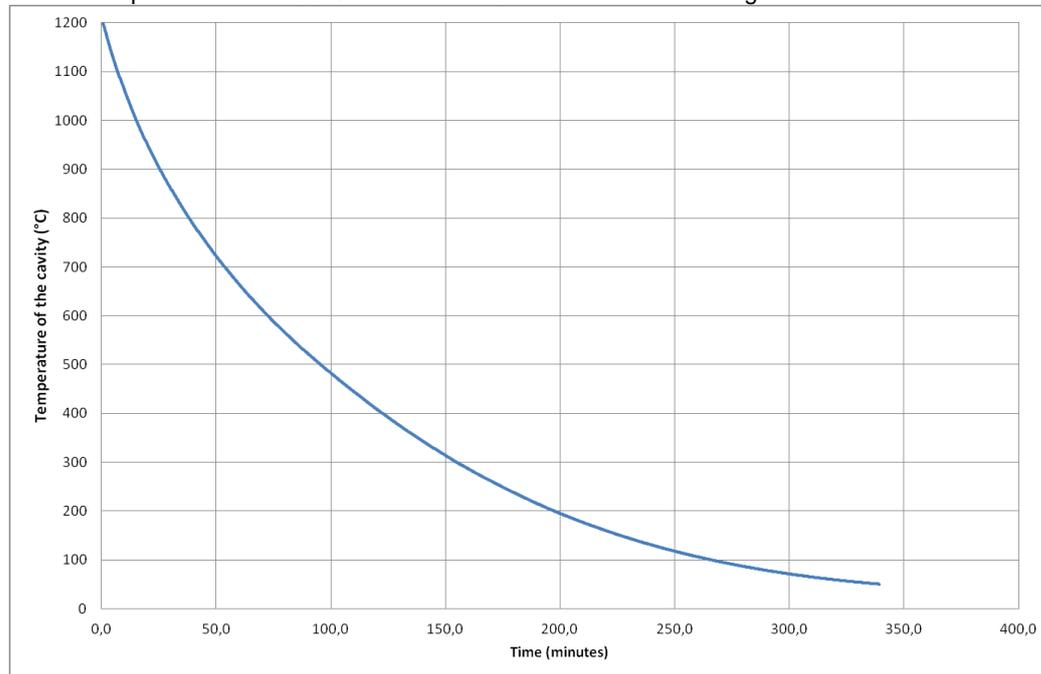
**Fig. 10:** Cooling curve of a cavity blackbody from  $1200^{\circ}\text{C}$
