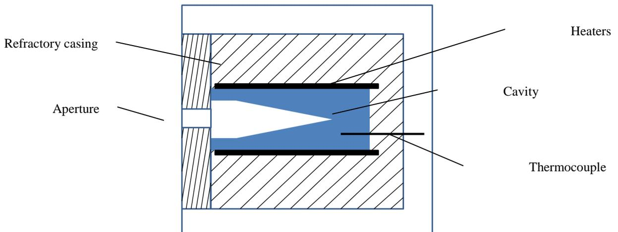
**Fig. 7:** cavity blackbody structure
