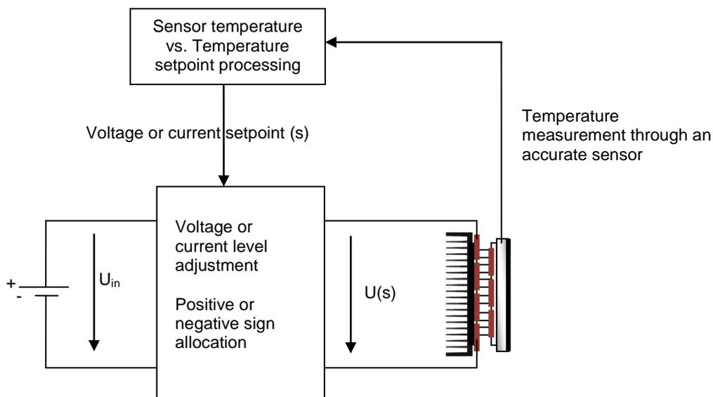
**Fig. 3.** Low temperature blackbody supply principle
