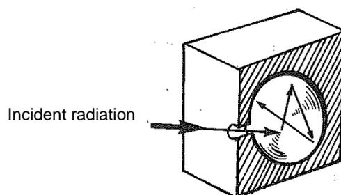
Fig. 6. Light trap principle
