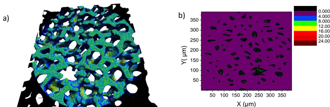
**Fig. 1.** Maps of radiative intensity of a  $\alpha$ -SiC foam with a size of  $12*12*2 \text{ mm}^3$  at  $T = 300 \text{ K}$  obtained with a Monte Carlo ray Tracing code, iMoorphRad [4, 5]: (a) 3D repartition of the reflected radiation (b) 2D repartition of transmitted radiation where white pixels correspond to the maximum of transmission
