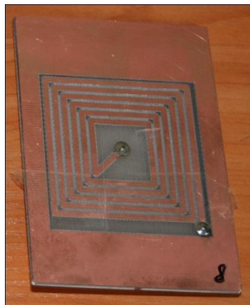
Fig. 6. 6-turn, 50 x 50 mm test spiral on 1.5 \mu\text{m} thick FR4 PCB (trace width - 1 mm, edge-to-edge segments distance - 1 mm, copper thickness 38 \mu\text{m} ).
