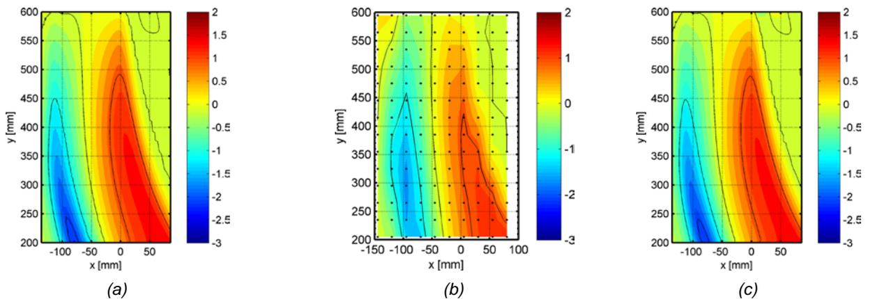
**Fig. 7.** Difference between the temperature map on the screen and the reference: homogeneous sheet with low in-plane conductivity (a); target net (b); cardboard screen (c).
