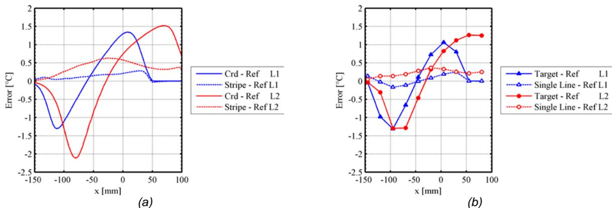
**Fig. 9.** Temperature difference, along L1 and L2, between the reference (Ref), the whole screen and the stripe/single line: cardboard (a); targets (b).
