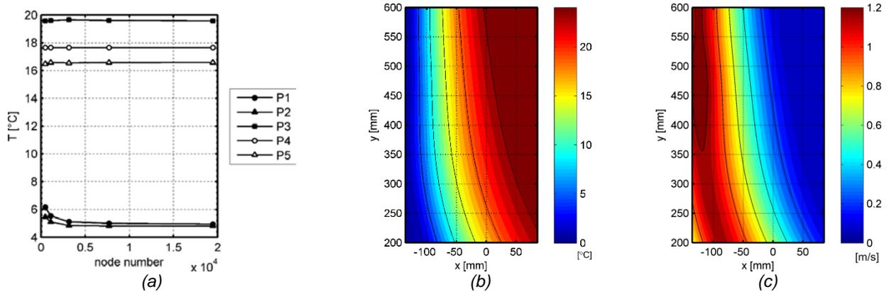
**Fig. 6.** Results of the sensitivity study (a); undisturbed temperature distribution on the symmetry plane (b) and the corresponding velocity field (c).
