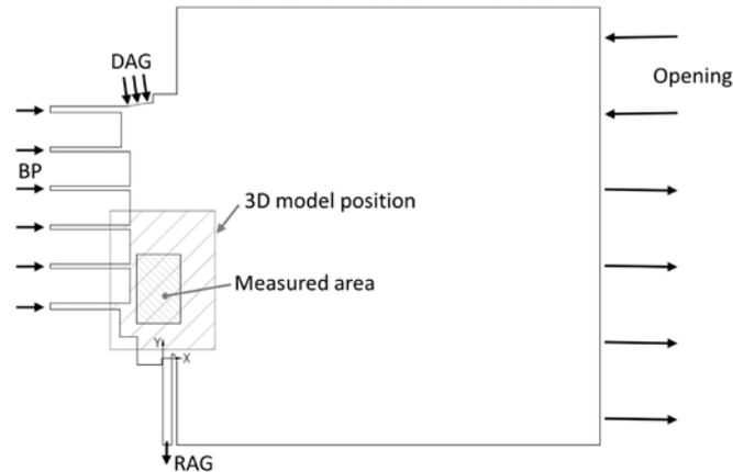
**Fig. 3.** Sketch of the ORDC 2D model with boundary and coordinate system.
