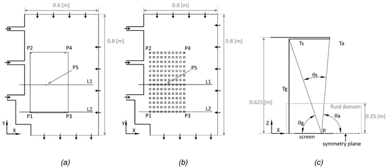
**Fig. 5.** Numerical model geometry and boundary; a) cardboard screen; b) net screen; c) sketch of the geometry used for the view factor calculation.
