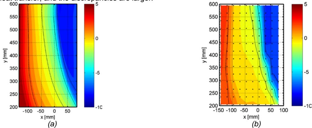
**Fig. 10.** Difference between the temperature map on the screen and the reference taking into account the radiative heat exchange: cardboard (a); targets (b).
