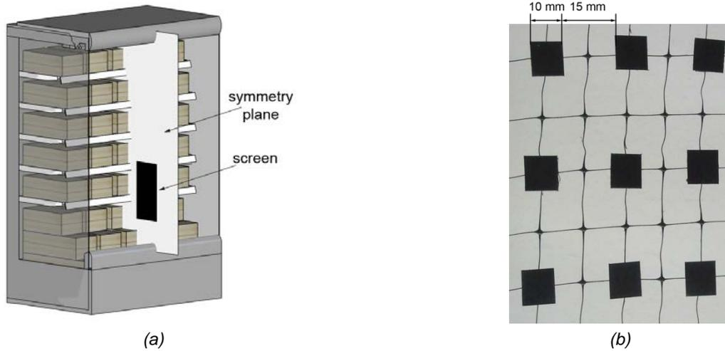
**Fig. 1.** Sketch of the experimental test (a); net with aluminium targets (b).
