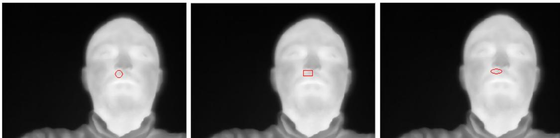
**Figure 1.** From left to right, circular, rectangular and Elliptic ROIs.
