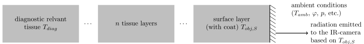
Fig. 3. Layer Model of the Surface Temperature Influences
