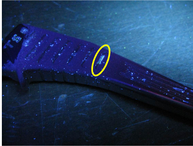
Figure 12: Inspection of a titanium prosthesis by penetrant testing
