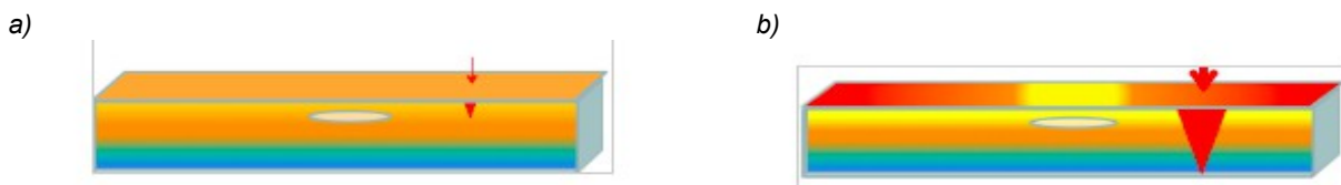
Fig. 9. Effect on surface when amplitude of stimulation is insufficient (a) and sufficient to detect the defect (b)
