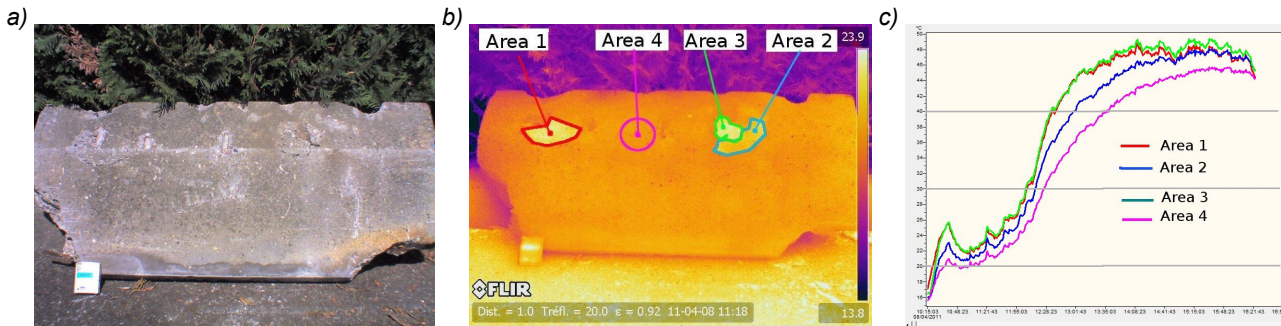
Fig. 6. Image of the sample of a bridge (a), infrared image with the 4 tested areas (b), mean temperature as a function of time for the 4 tested areas (c).
