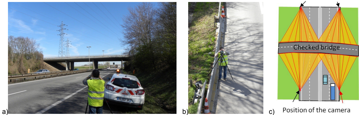
Fig. 14. Pictures of the camerawork (a and b) and implementation of shooting (c).
