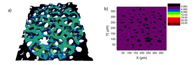
**Fig. 1.** Maps of radiative intensity of a  $\alpha$ -SiC foam with a size of  $12*12*2 \text{ mm}^3$  at T = 300 K obtained with a Monte Carlo ray Tracing code, iMoorphRad [4, 5]: (a) 3 D repartition of the reflected radiation (b) 2D repartition of transmitted radiation where white pixels correspond to the maximum of transmission
