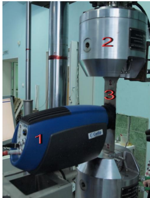
Fig. 2. Experimental setup (1 - infrared camera Flir SC5000, 2 – servohydraulic testing machine Bi-00-100, 3 - specimen).
