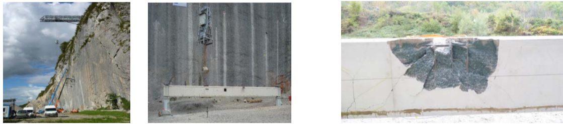
Fig. 4 IFSTTAR falling block test station (left), load of 2.5 T used (center), impact view (right)
